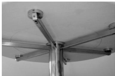
**3 |** Every precaution must be taken in the next step, that the outer table ring does not collide with the inner top (there is only a gap of 1 mm!) Lift the outer table top ring carefully over the inner table top plate and place it on the pedestal, that the 6 metal support parts are aligned with the 6 holes in the support arms of the pedestal. The markings on the metal support parts and on the 6 holes on the arms must match!
