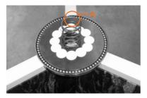
**1** I Place all precision balls into the groove of the turned center part and apply slightly some grease on the balls.
