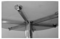
**3** I Every precaution must be taken in the next step, that the outer table ring does not collide with the inner top (there is only a gap of 1 mm!) Lift the outer table top ring carefully over the inner table top plate and place it on the pedestal, that the 6 metal support parts are aligned with the 6 holes in the support arms of the pedestal. The markings on the metal support parts and on the 6 holes on the arms must match!
