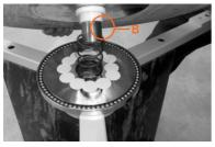
**2 I NOTICE** The table has been set in the factory and is marked with marking points on the table tops and at the base. Lift the inner table top carefully and evenly and thread the **ROD (B)** of the glued-on support part into the cylinder or socket of the pedestal.
