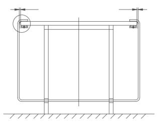
**3 I** Tighten the previously loosened grub screws with the plastic washers until the skids do not move any more.
