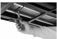
**5** I Lift the assembled pedestal at one side and remove both assembly stands. Cut-off both transport locks (cable straps) at the underside of the table.
