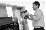
2 I Remove the 8 wood screws (Spax) according to the marking "♥" at the wooden bars of the transport box. ATTENTION Under no circumstances loosen the 4 cylinder head screws (see marked as "♥"), otherwise the extension frame will fall down in the box and will suffer irreparable damage!
