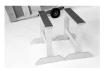
**1** I Position both assembly stands at the desired location of the table, that way, that the bases of the stands touch each other.
