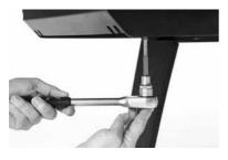
**12** I Now fully tighten both short countersunk screws M10  $\times$  30 mm and then the long ones M10  $\times$  55 mm at each main table top.
