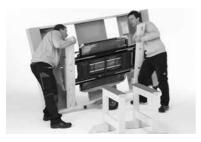
**3** I Raise the extension frame from the transport box and slew it from above with the connecting wood bars out of the box and place it carefully on the assembly stands.
