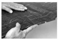
**11 I** Push all table tops firmly together and align the main table tops to the threefold extension. Please take care that you will have no gaps between the tops and no mismatches of the table top.
