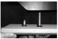
10 I Screw-in first the short countersunk screws M10 x 30 mm at the outer side of the frame, then the long countersunk screws M10 x 55 mm at the inner side of the frame, but not yet tighten them. SHORT for outside, LONG for inside Please continue the same way with the second main table top.
